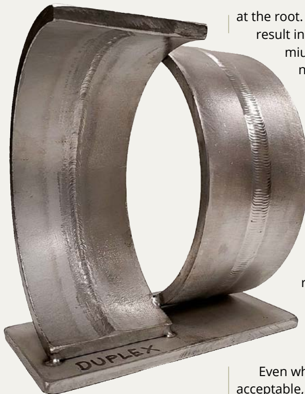
Cutaway weld specimen fabricated by Travis Field from 6" Schedule 40 duplex stainless steel pipe. The specimen was prepared to demonstrate weld penetration, bead profile, and welding execution capabilities to clients.
