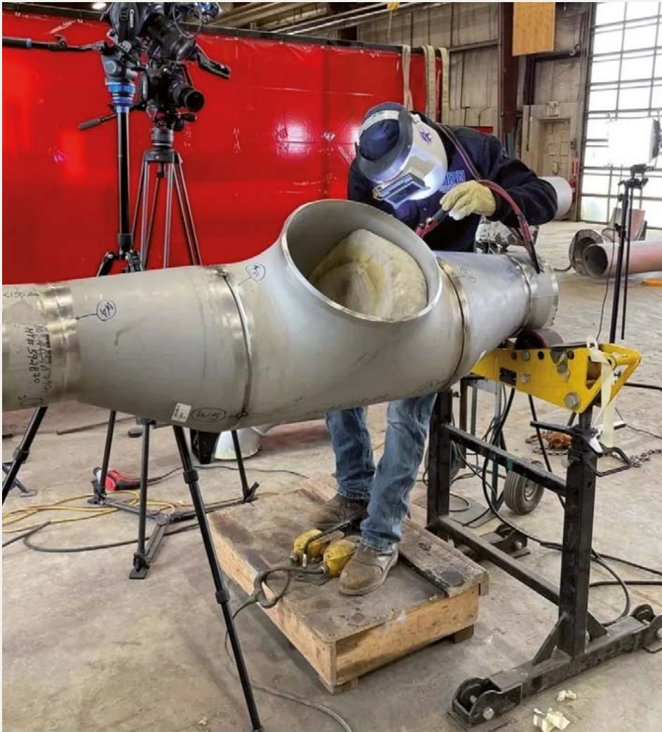
Travis Field performing GTAW welding on a duplex stainless steel pipe spool during filming for WeldTube educational training videos.
