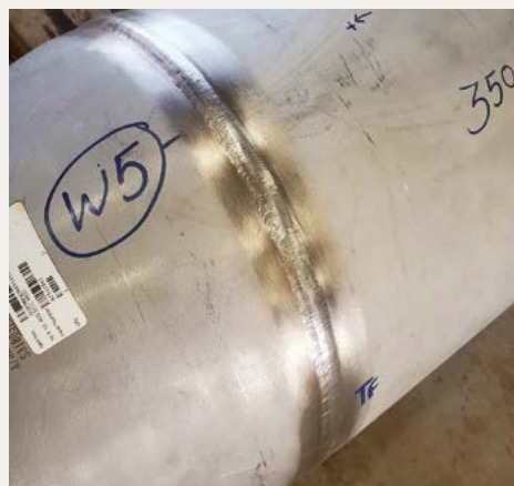
Duplex stainless steel pipe spool butt weld executed by Travis Field as part of production spool fabrication.
