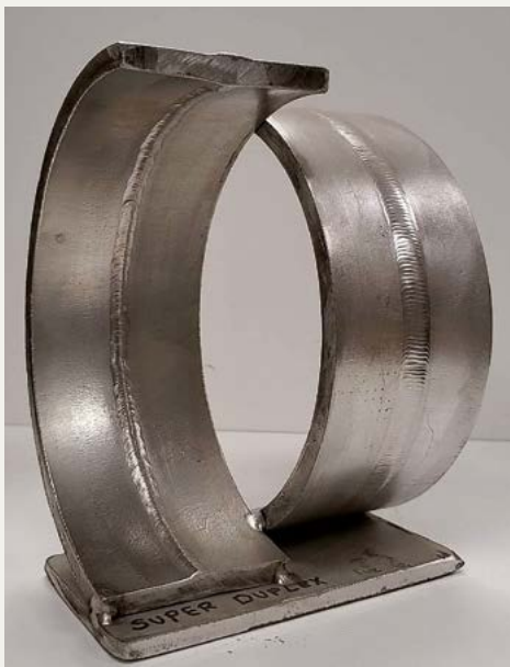
Cutaway weld specimen fabricated by Travis Field from 6" Schedule 40 super duplex stainless steel pipe. The specimen illustrates weld profile and execution quality in corrosion-resistant alloy piping systems.
