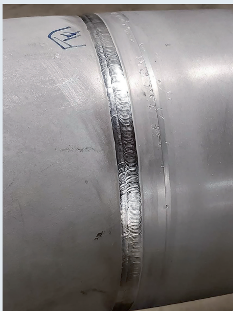
Completed external weld profile on 304H stainless process piping fabricated for elevated-temperature hydrocarbon or steam service.
