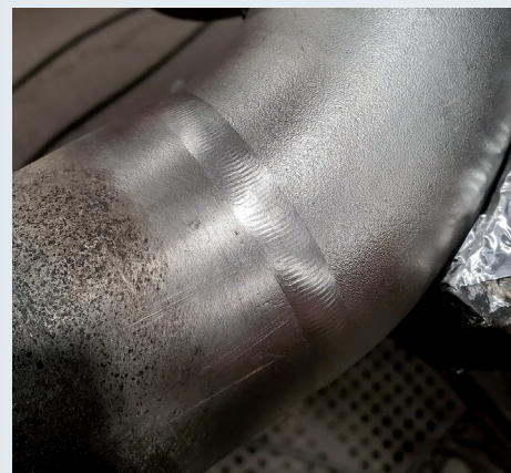
Finished weld on stainless process piping prepared for high-temperature service.
